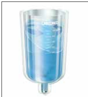
The gentle agitation of the sample tube causes the liquid to form a vortex-like configuration, which increases the sample's surface area and ability to evaporate.
